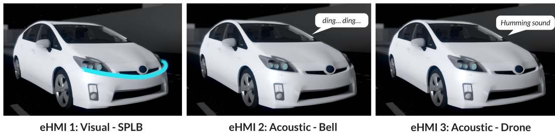
Fig. 1. We conducted a video-based study to test the effectiveness of 3 eHMIs: one visual (light-based: SPLB – Slow-Pulsing light Band), and two acoustic (sound-based: Bell eHMI that emits a dinging sound when the AV yields, and Drone eHMI that indicates a yielding intent by emitting a droning/ humming sound that changes pitch from high to low as the vehicle decelerates). Results showed that despite divergences in subjective opinions, the contrast between the eHMIs – individually or in combination with each other – had little effect in road-crossing decision objectively, indicating that once learned, eHMIs tend to work in general and design differences have relatively less impact. This leaves room for taking subjective user feedback into account in designing a pleasant user experience for eHMIs.
